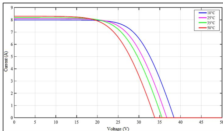
Figure 15: Characteristics I-V with the temperature variation
