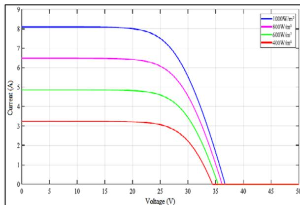
Figure 13: Characteristics I-V with the variation of solar irradiation
