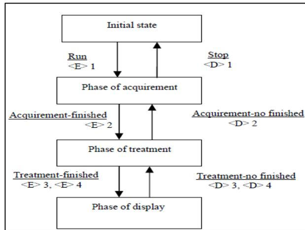
Figure 10: State - Transition diagram of the PV system
