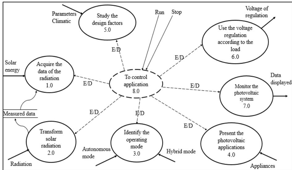
Figure 9: Control Flow Diagram of the PV system
