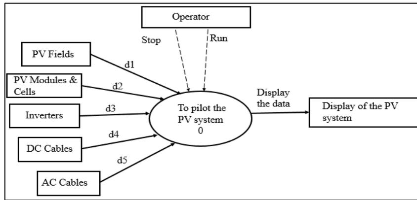
Figure 8: Context Diagram of the PV system
