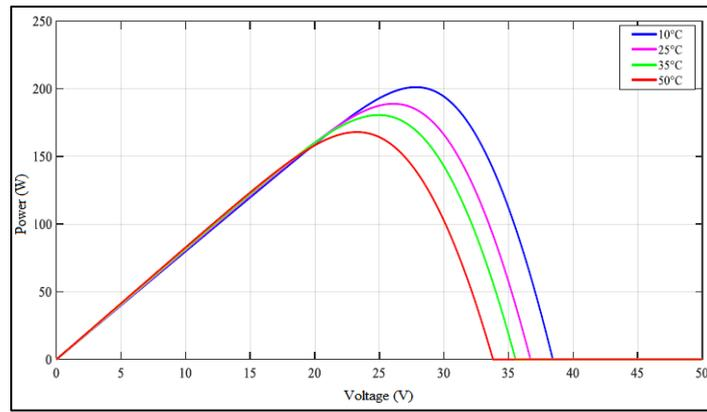
Figure 14: Characteristic P-V with the temperature variation
