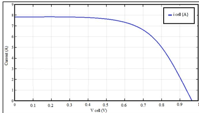
Figure 12: Current / voltage characteristic of a photovoltaic cell
