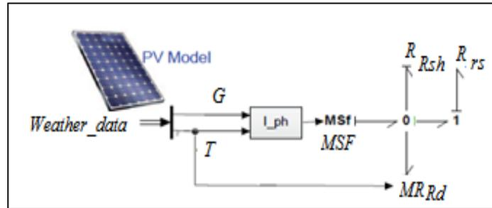
Figure 11: Bond graph model of the photovoltaic cell
